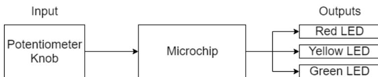
Figure 3 I/O Plan
